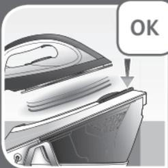
**During ironing, do not leave the iron on the soleplate or on the flush accessory. It is safe to leave the iron on the base of the steam generator or on the heel.**
