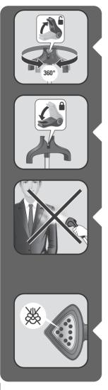
To release the hanger, unlock the lock system by pulling it up.
