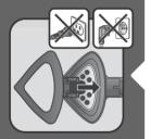
The crease attachment allows you to press a crease either on your trousers or jackets. Attach the crease attachment to the steam head when appliance is unplugged.
