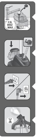
Unscrew the cap then fill the water tank with untreated tap water.
