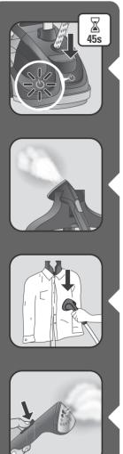
Press on the ON/OFF pedal and check that light is switching on. Wait for 45 seconds before steaming.
