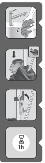
Unscrew the cap and then empty the water tank completely in a sink.
