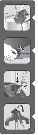
Vertically tilt the appliance to empty the water into the sink.
