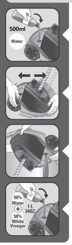
Pour 500 ml of water into the appliance tank inlet.
