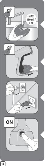
Fill the water tank with a maximum of EN 150 ml of untreated tap water.
