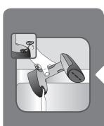
Empty the water tank completely and then close the water inlet cap.
