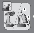
For storage purposes or to place in the travel pouch, it is possible to fold the appliance. Always press the head unlocking button before folding the head.
