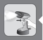
Press the steam button with the steam head facing away from you holding it in a vertical position.
